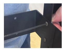
3. Tighten screws with Allen wrench as shown above.
