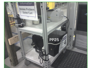
PP25 Stand Alone Power Package shown on bottom of cart
